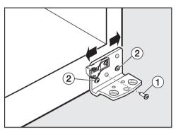
To align the **lower door** use the long outer slots in the lower hinge plate:
